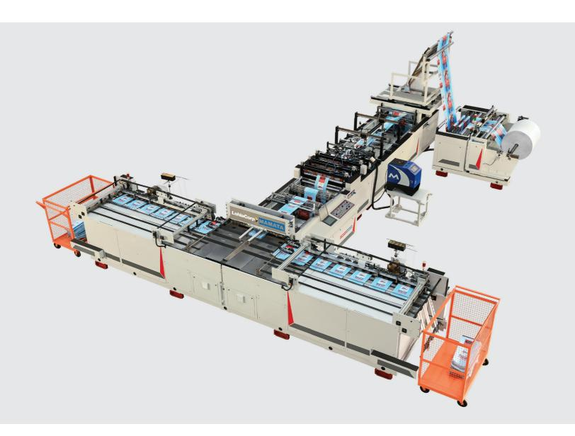
**LM-650** is the world's first high speed "Back Seam Sack" making machine from woven polypropylene tape fabric in flat form, laminated with reverse printed BOPP film, thereby giving a premium look for retail packaging. It is a compact machine equipped with integrated tubing and bag-making operations resulting in huge space savings.
