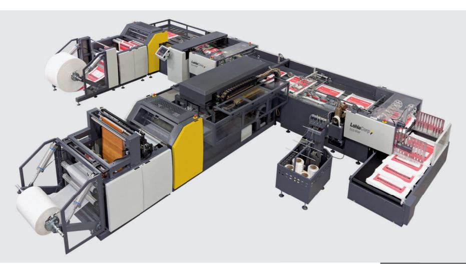
**bcs-liner** is the latest addition in our range of conversion machines. It automates and replaces the manual process of inserting liner in the woven bags. The machine uses PE/HDPE/LLDPE rolls which are cut at desired length, sealed and inserted in the woven bags. It is suitable for non-laminated fabric with an option for laminated fabric. These Liner bags are used in packaging of hygroscopic materials such as sugar, salt, chemicals & minerals.
