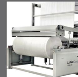
Magazine winder is recommended for winding heavy GSM tubular fabrics used for FIBC applications in which desired fabric tension can be adjusted by regulating torque through winder motor. The fabric roll is located above the ground level for ease of unloading with a forklift.
