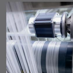
**Positive Warp In-feed System** having inlet motor with load cell control, regulates the tension of warp tapes on each inlet roller separately, by controlling its speed. Desired warp tension can be adjusted depending on fabric/tape specs. to improve fabric quality.
