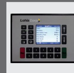
**Microprocessor Based Control System** is used for setting various machine & process parameters. Performance parameters such as Shift wise as well as cumulative production, efficiency, breakage as well as exhaustion incidents of warp & weft, roll length are updated/seen.
