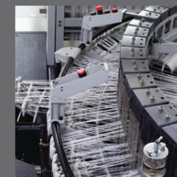
Separate re-inforcement blocks are mounted on compensation system for efficient production of FIBC fabric with re-inforcement strips.
